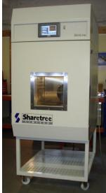
A general-purpose bench top chamber designed for Temperature/humidity Testing of PCB's and small assemblies.
