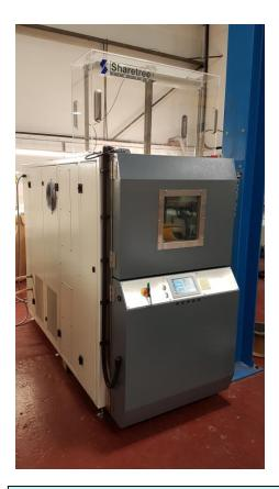
A specialist floor-standing chamber designed for Thermal Shock testing using two chambers, one hot and one cold, and a lift to move the products between them.
