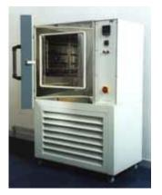
A general-purpose temperature cycling chamber with vertical airflow.
