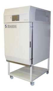
A general-purpose liquid nitrogen (LN2) cooled chamber designed for Thermal Testing of PCB's and small assemblies.
