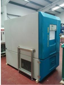
A general-purpose floor-standing chamber designed for Temperature testing.
