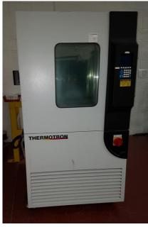
A 453litre temperature humidity chamber with cascade compressor cooling.
