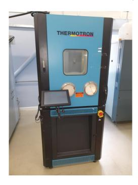
A 284 litre temperature humidity chamber with cascade compressor cooling.
